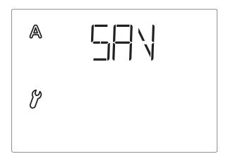
Press the SET key in order to save your entered data and to access the meteorological data display. With  $\Box$ , you quit the automatic settings without saving.
