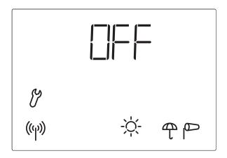
Leave this display at IFF if Arexa is used as conventional single-channel control system. The function "Sending of weather and automatic data" must only be activated if Arexa shall cooperate with motor control devices (e.g. XS MSG2-AP) in the control system XS.
