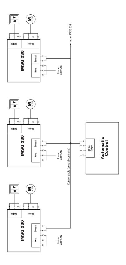
**Central control with group formation** with motor control units at the drive output of Arexa weather station:
