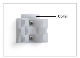
Fasten the mount vertically onto the wall or pole. When wall mounting: flat side on wall, crescent-shaped collar upward.
