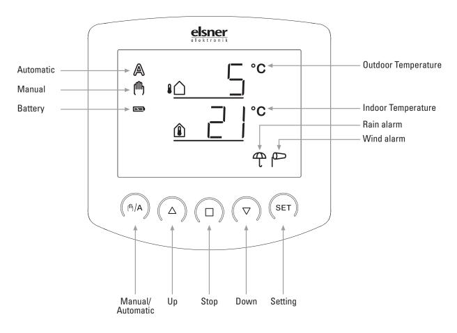
The basic position of the operating unit of the control system displays the current outdoor temperature (upper line) and the indoor temperature (lower line) as well as the function mode (automatic or manual), the battery load and the current alarm messages for rain or wind. The meteorological data are updated once per minute (and in case of a keystroke).
