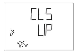
If the up and down connection cables have been mixed up when connecting the drive mechanism, this may be corrected in this step. First open the window a little bit for the rotational direction test. Check both arrow keys and make a setting in the display, whether the window closes again with  $\nabla$  or with  $\triangle$ .
