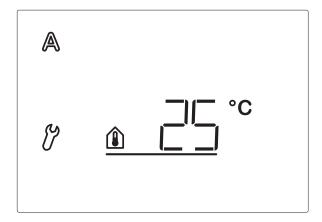
As soon as the value indicated here is exceeded, the automatic opens the window (unless the blocking value for the outdoor temperature has fallen below, see next parameter). The delay (hysteresis) is 2°C. That means, that the window will be closed as soon as the indoor temperature drops 2°C below the set value.
